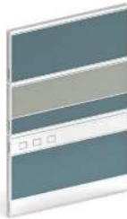
BELOW IS FABRIC PANEL, ABOVE IS FABRIC WITH TWO MAGNETIC PANEL AND BELOW WORKSURFACE POWER ACCESS AND LOWER RACE-WAY
